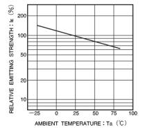
Fig.4 Relative emitting strength vs. ambient temperature
