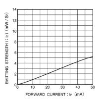
Fig.3 Emitting strength I vs. forward current
