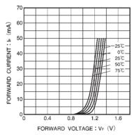
Fig.2 Forward current vs. forward voltage
