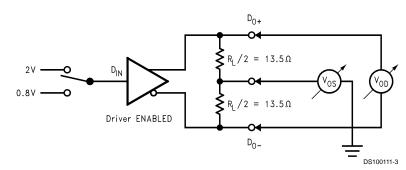
FIGURE 1. Differential Driver DC Test Circuit
