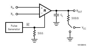
FIGURE 8. Receiver TRI-STATE Delay Test Circuit
