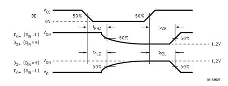
FIGURE 5. Driver TRI-STATE Delay Waveforms
