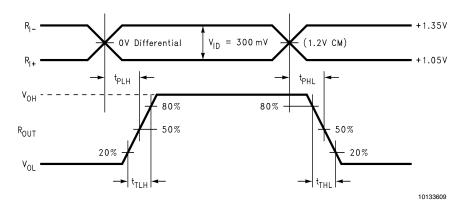
FIGURE 7. Receiver Propagation Delay and Transition Time Waveforms
