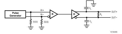
FIGURE 4. LVDS Output Load
