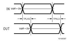
FIGURE 6. Propagation Delay Low-to-High and High-to-Low
