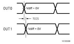
FIGURE 7. Output Channel-to-Channel Skew in 1:2 splitter mode
