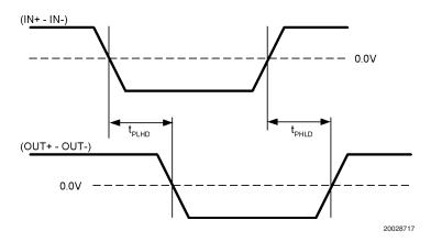
FIGURE 7. LVDS Output Propagation Delay
