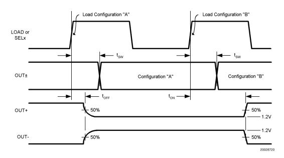
FIGURE 10. Configuration and Output Enable/Disable Timing
