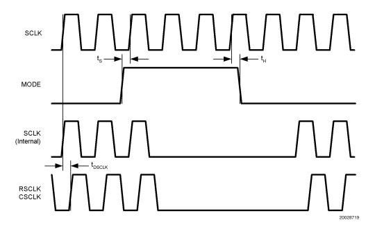
FIGURE 9. Serial Interface — MODE Timing and Functionality
