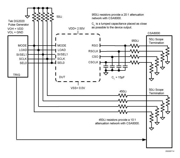
FIGURE 4. LVCMOS Driver AC Test Circuit (Note 6)
