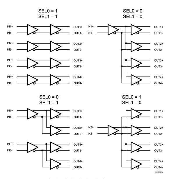
FIGURE 1. DS90CP04 Configuration Select Decode
