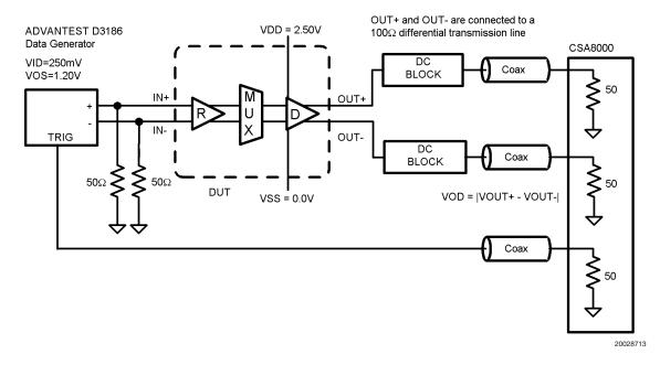
FIGURE 3. Differential Driver AC Test Circuit
