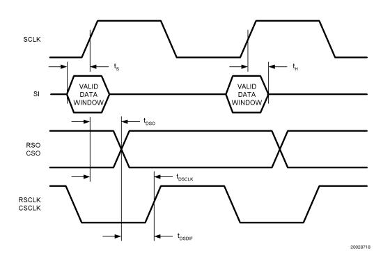
FIGURE 8. Serial Interface Propagation Delay and Input Timing Waveforms
