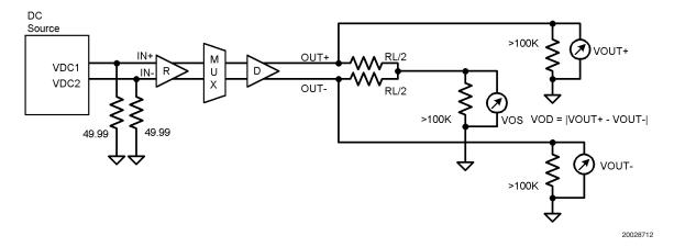
FIGURE 2. Differential Driver DC Test Circuit
