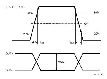
FIGURE 6. LVDS Output Transition Time
