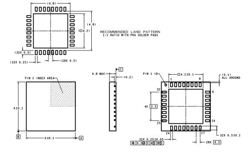
DIMENSIONS ARE IN MILLIMETERS
