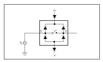
Figure 1. Overvoltage Protection Using External Blocking Diodes
