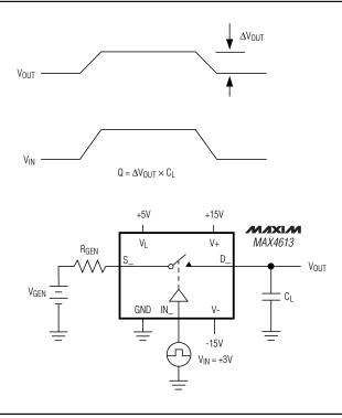
Figure 4. Charge Injection
