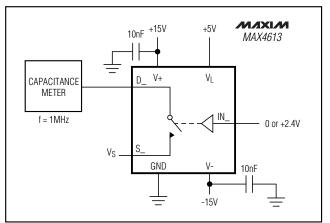
Figure 8. Source/Drain-On Capacitance
