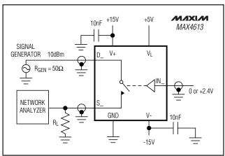
Figure 5. Off-Isolation Rejection Ratio
