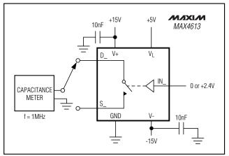
Figure 7. Source/Drain-Off Capacitance
