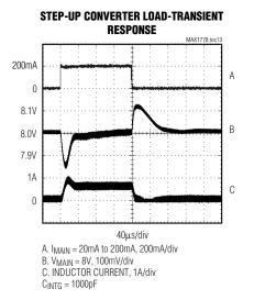
**STEP-UP CONVERTER LOAD-TRANSIENT RESPONSE WITHOUT INTEGRATOR** 200mA А 0 8 1 V В 8.0V 7.9V 1A С 0 40µs/div A. I<sub>MAIN</sub> = 20mA to 200mA, 200mA/div B. V<sub>MAIN</sub> = 8V, 100mV/div C. INDUCTOR CURRENT, 1A/div INTG = REF
