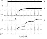
A.  $V_{\overline{SHDN}} = 0$  TO 2V, 2V/div B.  $V_{LDOOUT} = 5V$ ,  $R_{LDOOUT} = 125\Omega$ , 2V/divC.  $V_{MAIN} = 8V$ ,  $R_{MAIN} = 40\Omega$ , 2V/div
