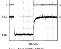
A. ILDO = 100µA TO 40mA, 40mA/div B. V<sub>LD0</sub> = 5V, 20mV/div  $V_{IN} = V_{LDO} + 100 \text{mV}$
