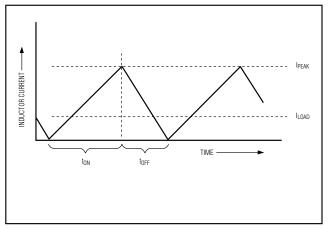
Figure 3. Discontinuous-to-Continuous Conduction Crossover Point
