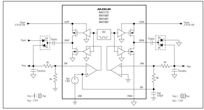
Figure 4. Low-Power Charge Pump Block Diagram
