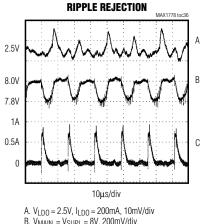
A.  $V_{LD0}$  = 2.5V,  $I_{LD0}$  = 200mA, 10mV/div B.  $V_{MAIN}$  =  $V_{SUPL}$  = 8V, 200mV/div C.  $I_{MAIN}$  = 0 T0 750mA, 500mA/div FIGURE 7
