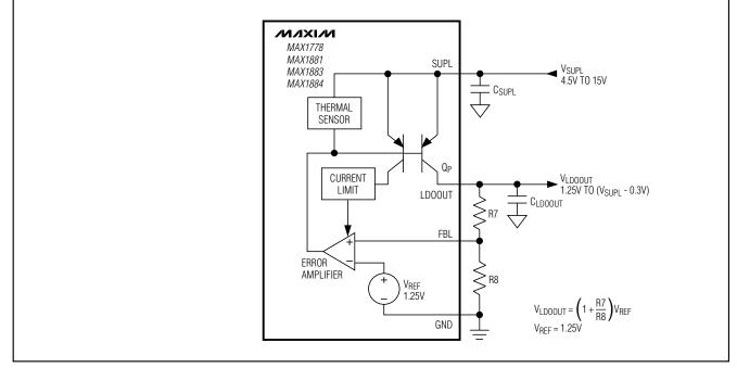
Figure 5. Low-Dropout Linear Regulator Block Diagram
