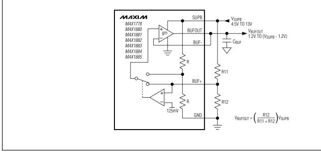
Figure 6. VCOM Buffer Block Diagram
