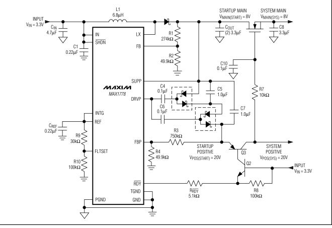
Figure 10. Power-Up Sequencing and Fault Protection;
