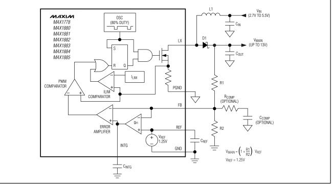
Figure 2. Main Step-Up Converter block Diagram
