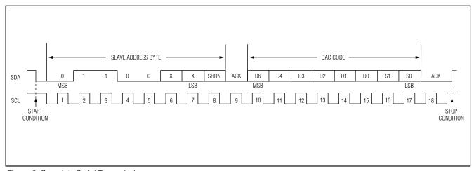
Figure 6. Complete Serial Transmission
