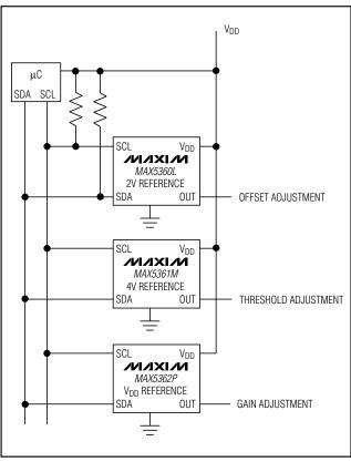
Figure 7. I<sup>2</sup>C Typical Application
