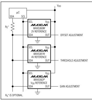
Figure 4. Typical Application Circuit
