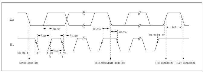
Figure 3. Two-Wire Serial Interface Timing Diagram
