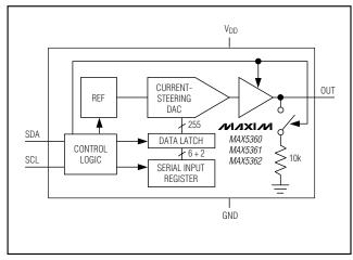
Figure 1. Functional Diagram
