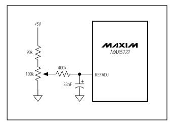
Figure 3a. MAX5122 Reference Adjust Circuit
