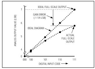
Figure 8d. Gain Error
