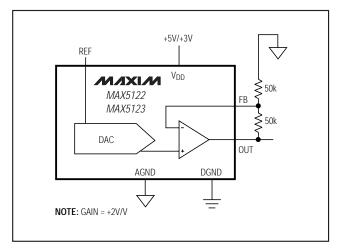
Figure 9. Unipolar Output Circuit Using Internal (+1.25V/+2.5V) or External Reference. With external reference, pull REFADJ to Vpp.
