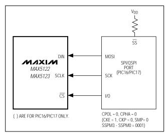
Figure 4. SPI/QSPI Interface Connections (PIC16/PIC17)
