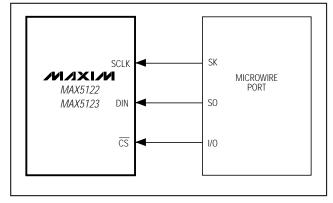
Figure 5. MICROWIRE Interface Connections
