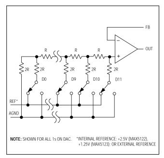
Figure 2. Simplified Inverted R-2R DAC Structure
