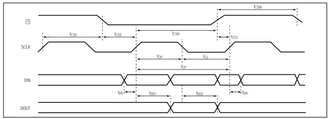
Figure 7. Detailed Serial-Interface Timing
