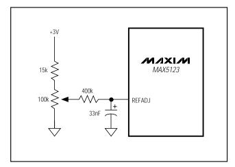
Figure 3b. MAX5123 Reference Adjust Circuit
