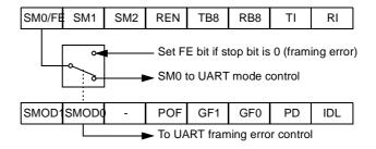
When this feature is enabled, the receiver checks each incoming data frame for a valid stop bit. An invalid stop bit may result from noise on the serial lines or from simultaneous transmission by two CPUs. If a valid stop bit is not found, the Framing Error bit (FE) in SCON register bit is set.
