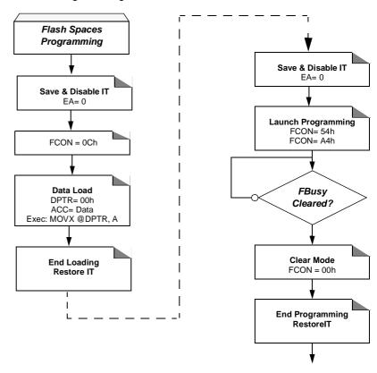
Figure 14. Hardware Programming Procedure
