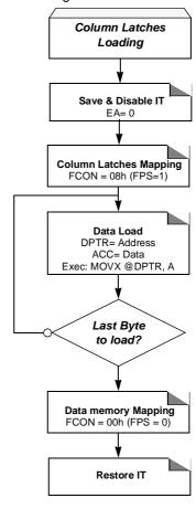
Figure 12. Column Latches Loading Procedure
