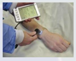
Adding data to or retrieving data from a patient's personal credential is simple and unobtrusive by using integration packages like those offered by One Touch Technologies. Unlike chip-based cards, <u>i</u>Buttons can easily attach to wristbands, rings, watches, or other commonly worn items. The stainless-steel encased <u>i</u>Button protects critical data from exposure to liquids, chemicals, body fluids, and other destructive elements.
